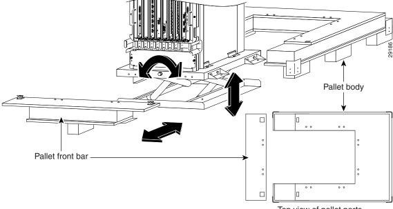
To reinstall the router and scissor-jack platform on the shipping pallet, use Figure A-7 as a reference and follow these steps:
